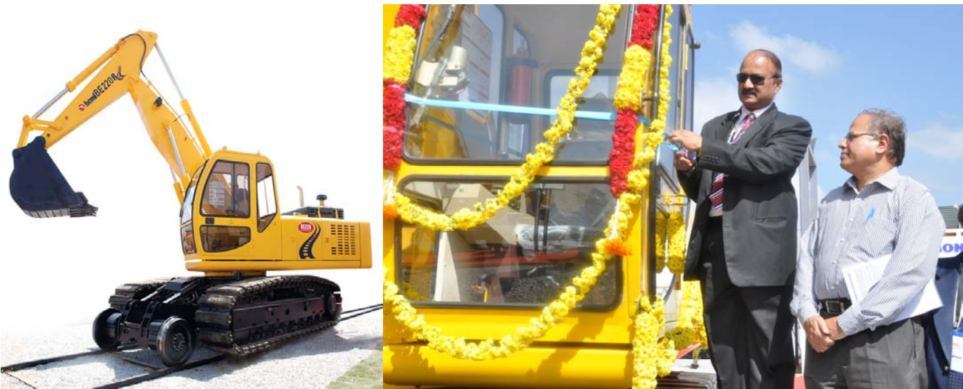
The twin purpose construction equipment BE220R that Performs on both Rail & Road
